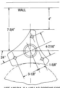
USE 1/2" DIA. X 1-1/2" LAG SCREWS FOR **FASTENING TO FLOOR**
