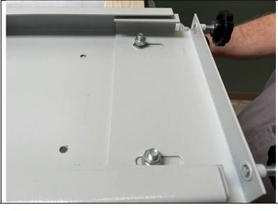
Place mounting plate on top and adjust railing for fitment
