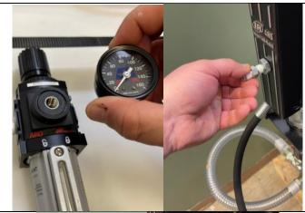
Attach the Regulator to the pump
