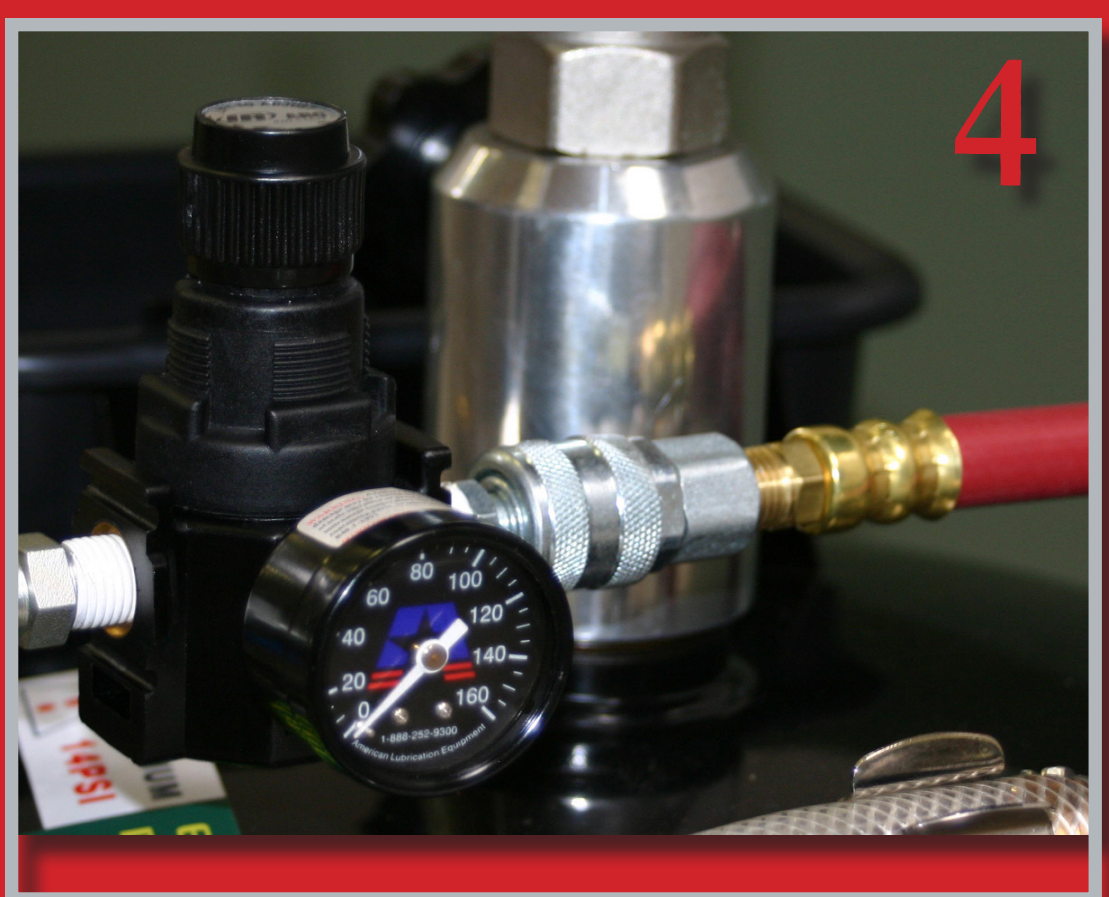
4 Make sure air pressure regulator is set to 7 PSI
