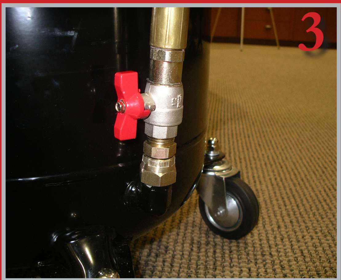
3 Open material outlet shut off valve at the base of the drain.
