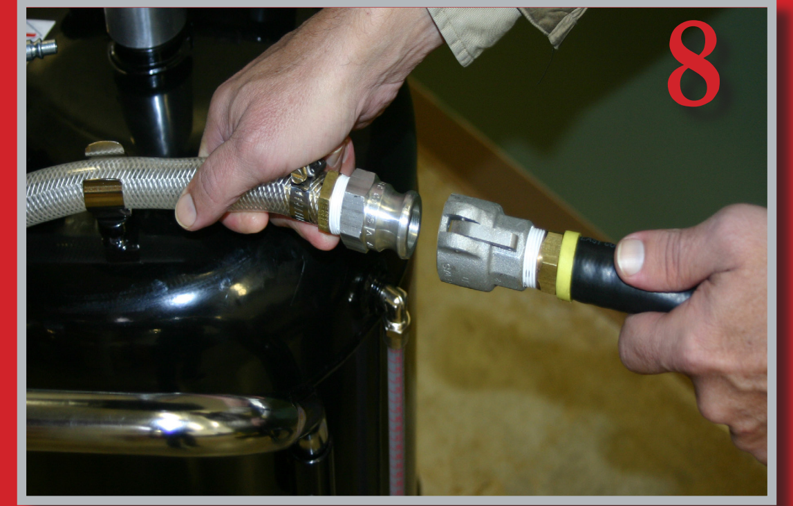
8 Disconnect fluid coupler on the waste oil tank inlet hose from the fluid connector on the drain.
