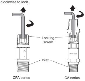
5. Verify cracking pressure.
