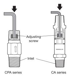
3. Turn both screws clockwise to increase cracking pressure, counter-clockwise to decrease.
