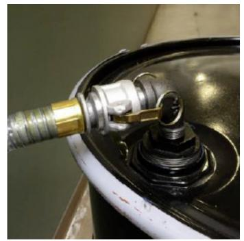
Screw and tighten 3/4" 90° swivel end of TIM-730-1 suction hose into pump inlet. This fitting must be taped, and pipe doped.
